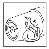
The Forward Collision Alert (FCA) controls are located on the end of the multifunction lever.
